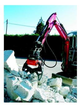
The model 430 DE T34 concrete crusher is designed to suit smaller excavators, being most useful in demolition applications were smaller excavators can be used in confined spaces with limited access. The unit allows the crushing of concrete and masonry walls up to 430mm in thickness, which allows demolition to be accomplished with little noise, dust and vibration to the work areas environment.
