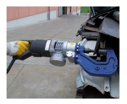
The Edilgrappa PG22/120DE electric hydraulic hole puncher is a precision made portable puncher that can be applied to any working position in any given environment, which allows the operator more flexibility to punch holes in confined situations for a wide range of applications. The PG22/120DE can punch through 6mm (250 Grade) mild steel plate maximum thickness.
