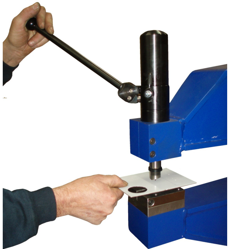
Centre Pin Adaptor – Extremely Accurate Hole Positioning
