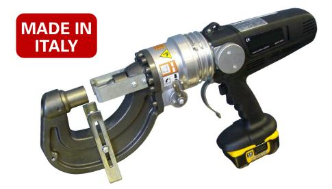
The PG22/60 DE cordless hydraulic hole puncher is a precision made portable puncher that can be applied to any working position in any given environment, which allows the operator more flexibility to punch holes in confined situations for a wide range of applications. The PG22/60 DE can punch through 6mm (250 Grade) mild steel plate maximum thickness.
