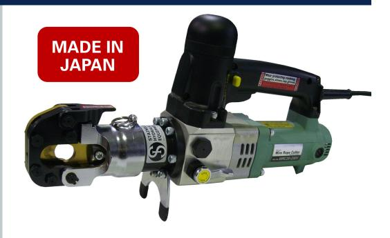
The WRC20 electric cable cutting range is designed to cut 20mm steel strand cable, steel core wire rope & insulated copper cable. These tools feature premium powdered high speed steel cutting blades with titanium coating for better blade longevity.
